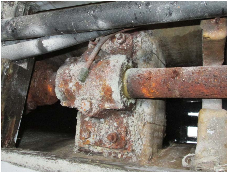
Photograph 26 - Intermediate shaft bearing
