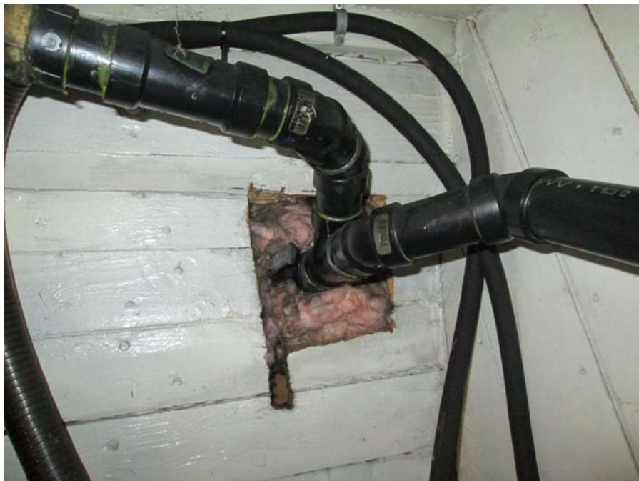
Photograph 22 - Bilge and grey water overboard discharge
