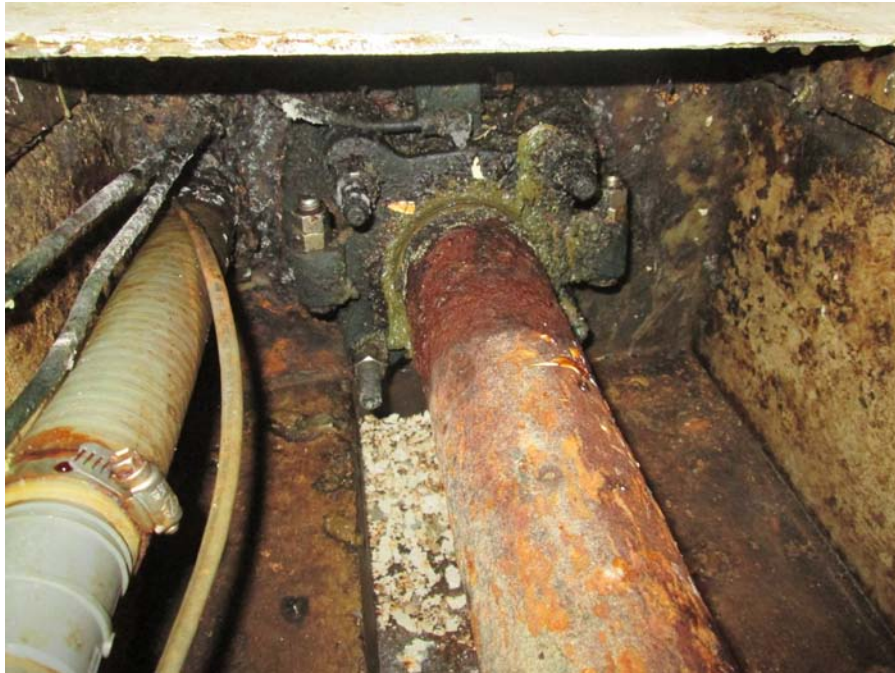
Photograph 27 - Shaft penetration at aft engine room bulkhead
