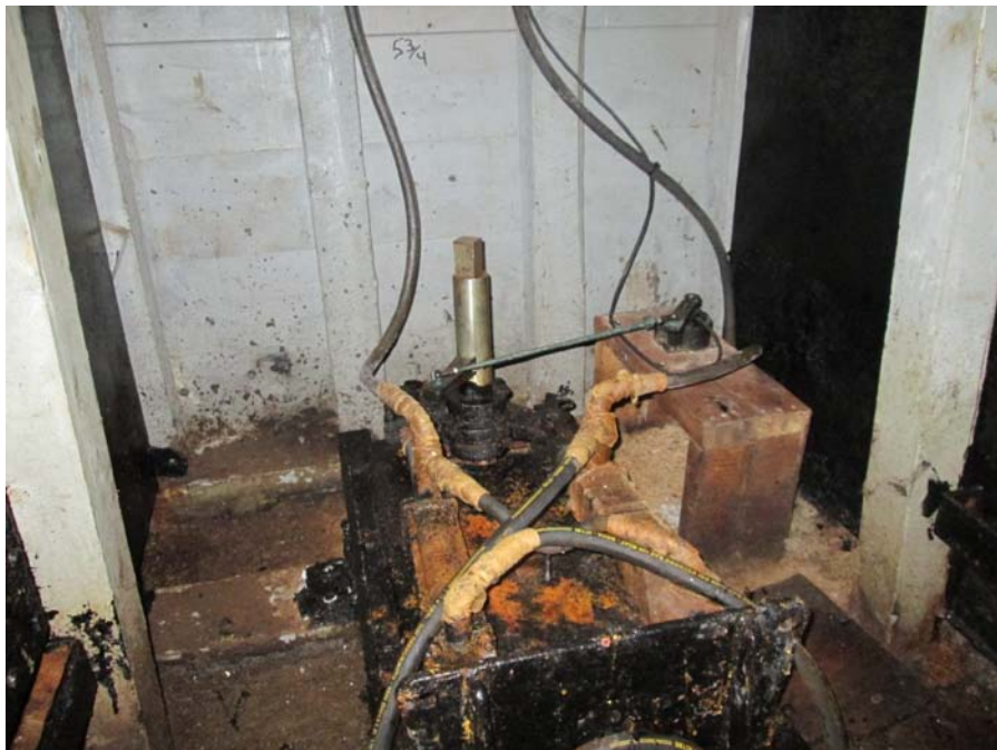
Photograph 24 - Hydraulic steering Gear
