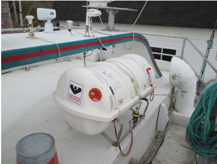
Photograph 27 - 8 person life raft on wheelhouse top
