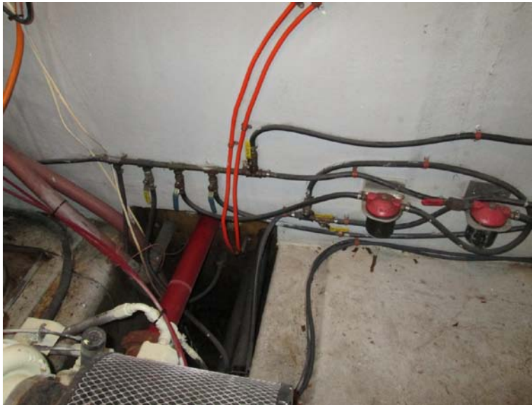
Photograph 17 - Fuel manifold and filters
