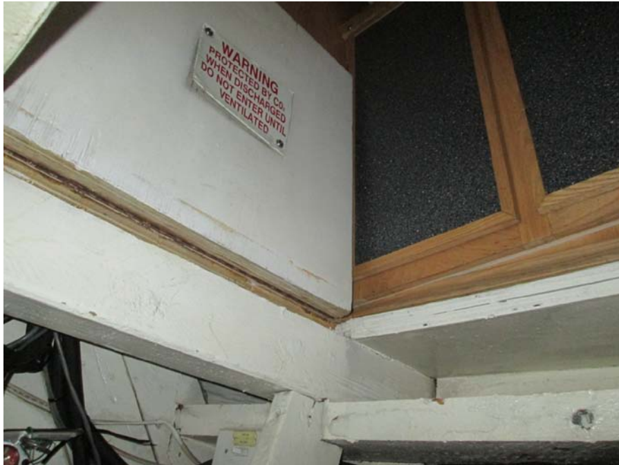
Photograph 23 - Engine room hatch. Note not gas-tight
