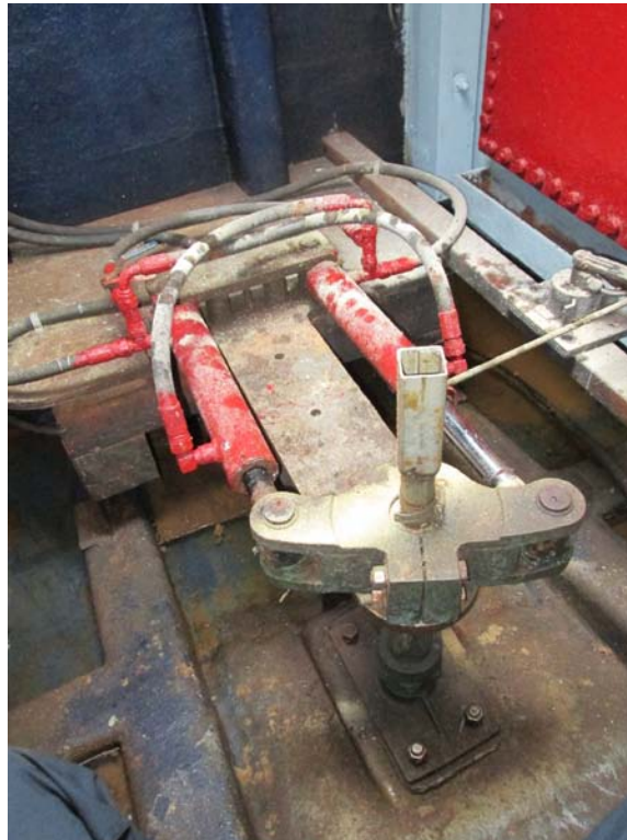
Photograph 12 - Steering Gear
