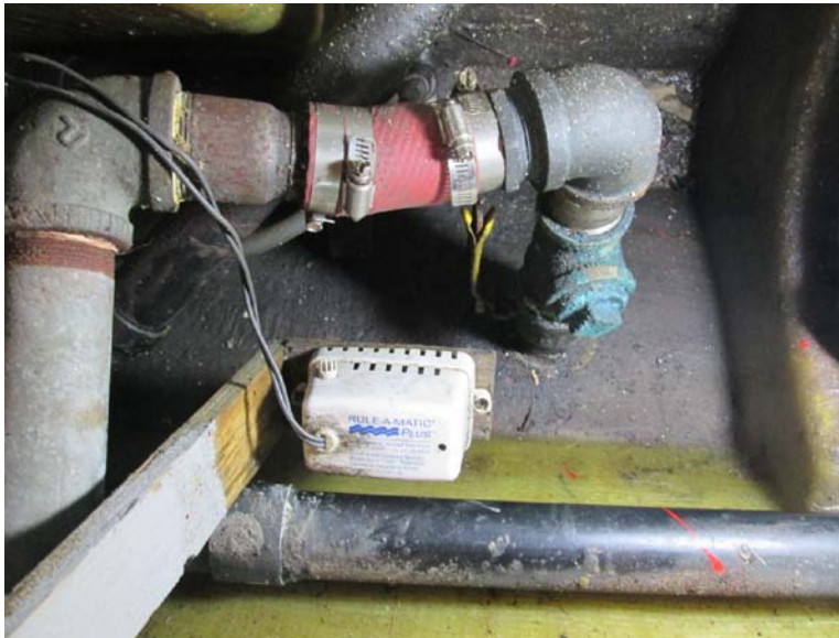
Photograph 18 - Salt water intake, engine room forward
