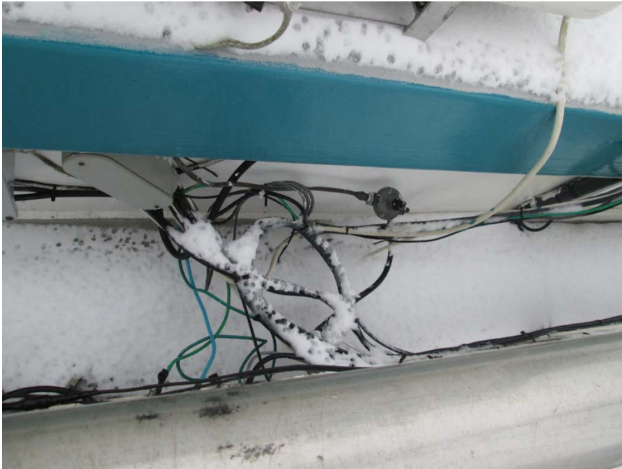
Photograph 13 - Propane connection on wheelhouse top
